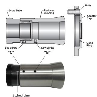
**Note:** There are four slots milled on the O.D. of the Draw Tube. Four corresponding lines are etched on the O.D. of the draw tube to indicate the location of each of the milled slots.
