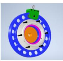
12) Remove 3 screws from ring and chuck body13) Slide the tool off from chuck body
