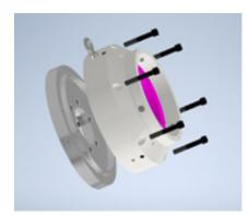
I) Remove chuck from packaging2) Unbolt the mounting plate from chuck
