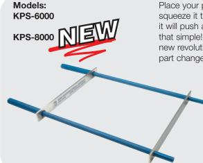
Place your parallels in the vise against the jaws. Take the Parallel Keeper, squeeze it together and place it inside the parallels. Release the Parallel Keeper, it will push against the parallels, holding them against the jaws of the vise. It's that simple! KPS-6000 model opens to 6". KPS-8000 model opens to 8". Your new revolutionary labor saver, your "machinists third hand," is at work, saving part change time. 1 lb. shipping weight.
