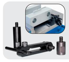
New adjustable workstop can be used on all Kurt high-density vises. The body clamp has a 2" adjustment and features a 3" long stop pin for fast and easy setups. A long and short spacer is also available to fit almost any application.
